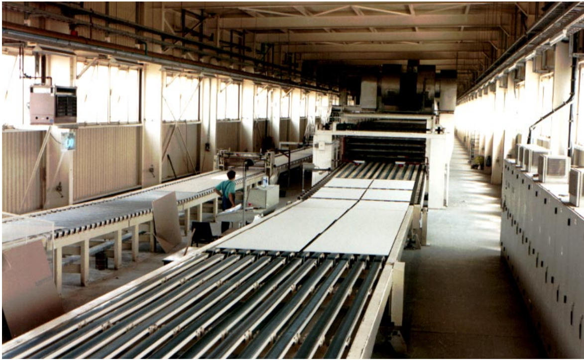
Manufacture of gypsum wallboard is highly automated
