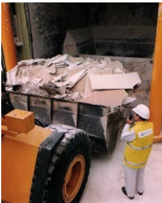
Waste gypsum wallboard being loaded into the reclamation plant
